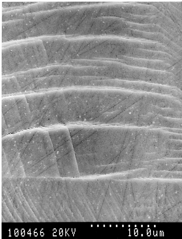
Figure 5 Electron micrograph of cracks in zirconia film above slip band region of 316L stainless steel.
